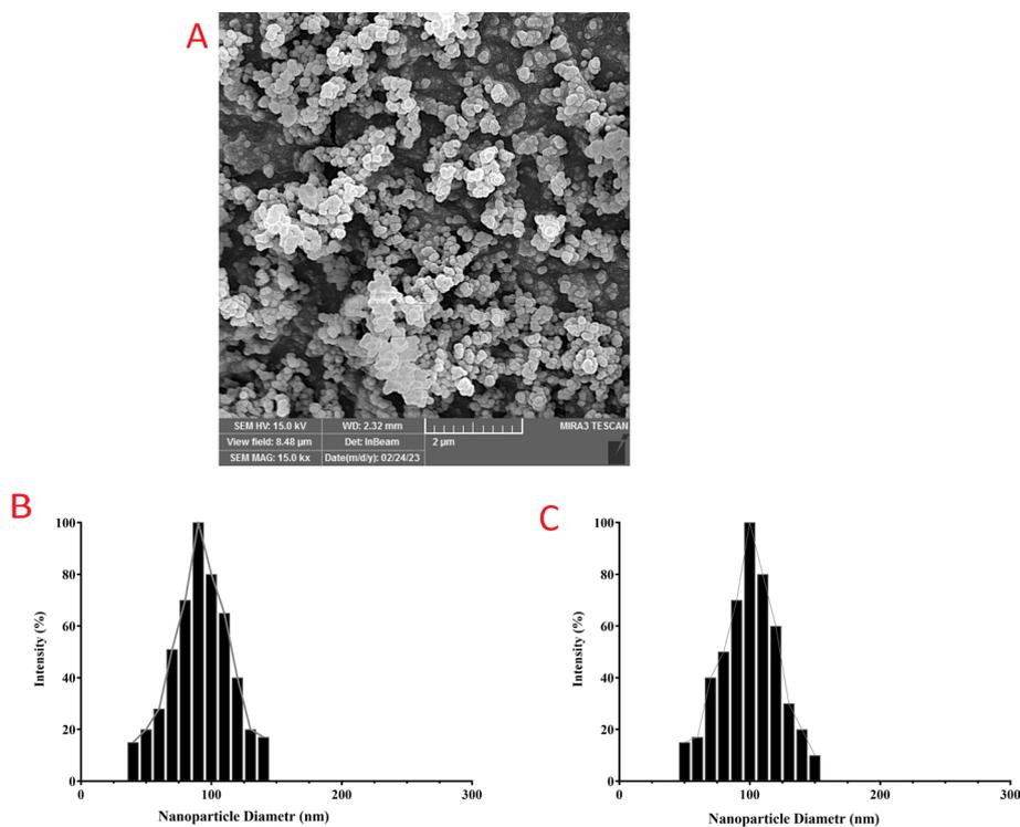
**Fig. 3** Characterization of the prepared MSNs. FE-SEM image of Art@MSNs (a). The DLS analysis on mean diameter of Art@MSNs (b and c). Results are mean  $\pm$  SD (n = 3)
