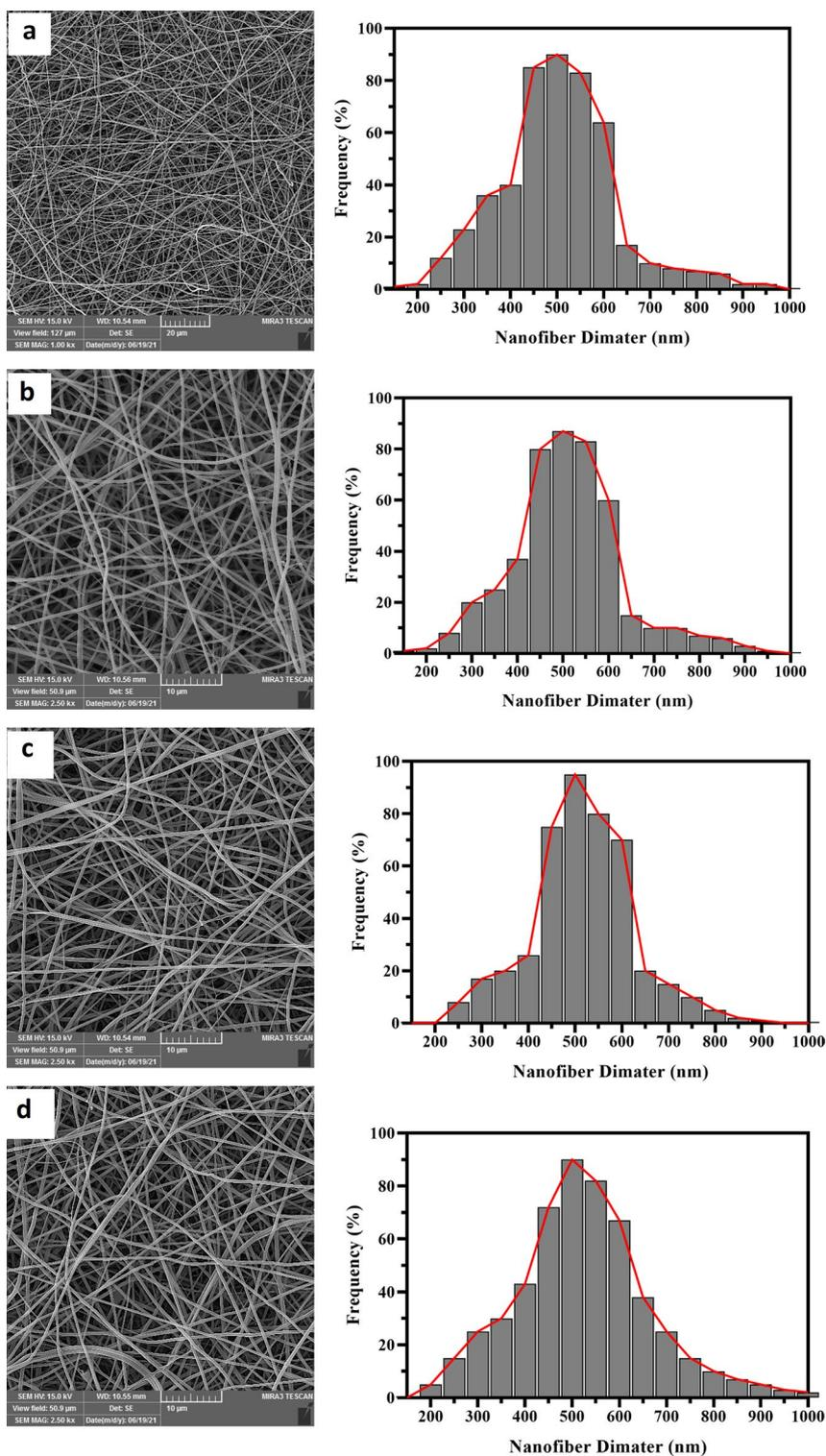
**Fig. 4** Morphological features of the fabricated composite NFs. FE-SEM micrographs of neat NFs (a), Art-NFs (b), MSNs-NFs (c), Art@MSNs-NFs (d). These results are representative of  $N = 3$  with similar outcomes
